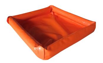
Designed with low-profile foam sidewalls (typically 2–4 inches / 50–100 mm high), these berms allow for easy drive-in and drive-out access while maintaining reliable containment of hazardous liquids such as oil, fuel, and chemicals.
