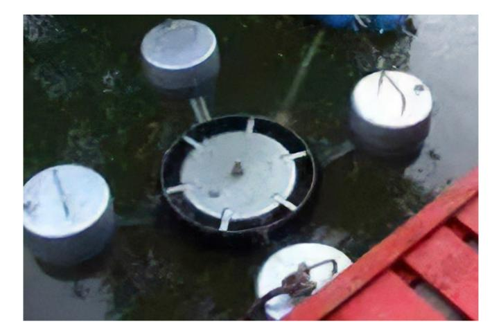
AQUA skimmers can be installed with booms during OSR operations. Also intended for stationary use in sedimentation tanks, tanks.
