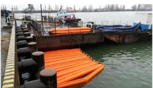
Boom barriers are equipment used for the localization, movement, and collection of oil products during emergency oil spills.
