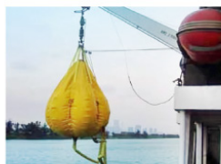
5 Proof Load Testing
