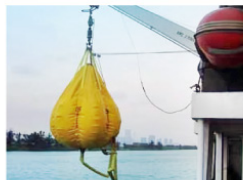
5 Proof Load Testing
