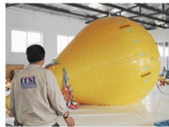
3 Air Tightness Inspection
