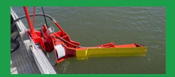
Minibagger is a highly effective, cost-effective, rapid response tool for localized oil spills in coastal areas, lakes, and ports and marinas
