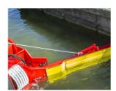
Skimmers, oil skimmers - mechanical equipment for the removal of oil, grease and oil products from the surface of water, coolant, emulsions, washing solutions, waste water.
